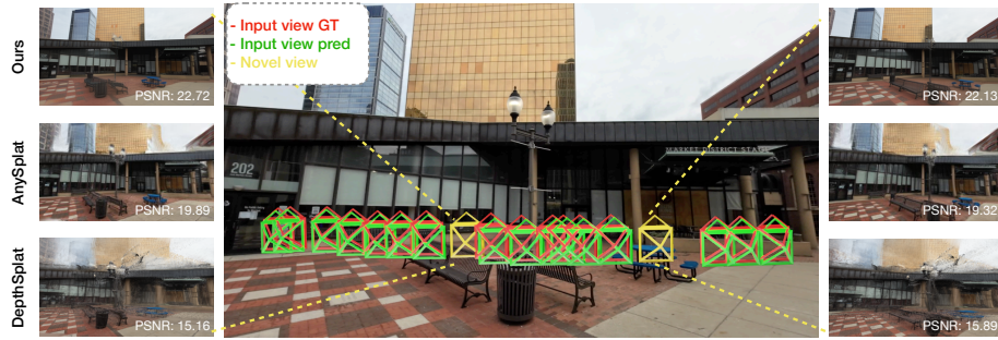
Fig. 1: LVSPM can jointly achieve high-quality novel view synthesis and accurate camera pose estimation from uncalibrated long-sequence (128) multi-view images. A subset of the 128 input views with corresponding prediction and ground-truth poses is shown in the middle, while novel view synthesis comparisons are presented on the side. Our estimated poses closely align with ground truth, while our pose-free synthesis results surpass recent baselines, including the pose-free AnySplat [26] and even the pose-required DepthSplat [72].
